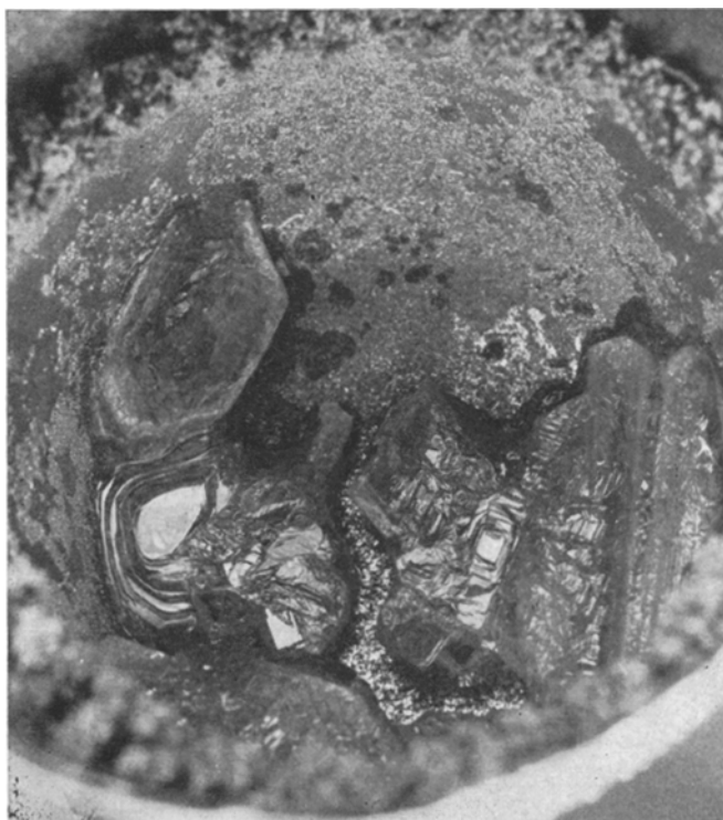
Figure 1 Crystals of Yb_2Ge_2O_7 , at the base of a 1.5 cm diameter crucible, after evaporation of PbF_2 .
